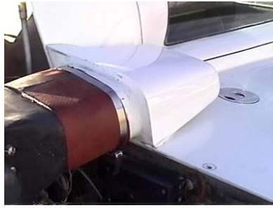
A custom made BID duct joins the intake to the plenum.
