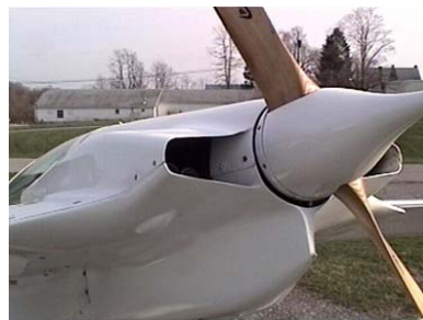
Exhaust pipes end three inches inside the cowling.
